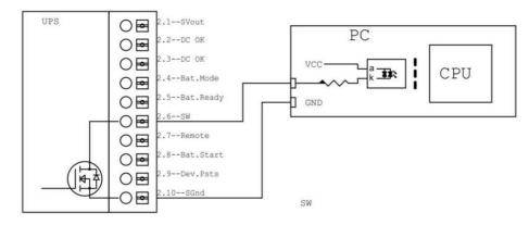
When the AS56UPS001 works in the load current monitoring mode, if the load current is lower than the set threshold (set by the rotary switch), the SW will output a pulse signal, whose pulse width time\_h can be set by Modbus register 40013.
